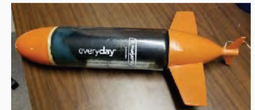
Lead Zeppelin: 1/3 scale model of Deepglider Soon to be upgraded to clear cylindrical body.
